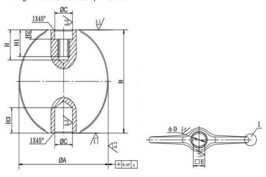
Drawing of center-line butterfly valve disc:
